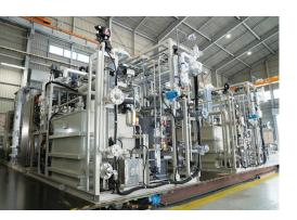
De Nora CECHLO-MS-200 on-site generator uses the general world-proven ion exchange membrane electrolysis process to generate high concentration sodium hypochlorite of 12% and/or chlorine gas. At the heart of the CECHLO-MS 200 system is the highly efficient proprietary electrolyser, continuously improved through innovative upgrades.
